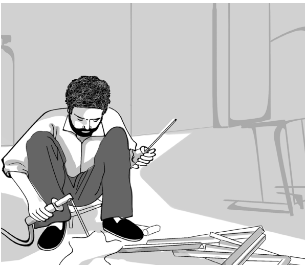
3. Not providing welding helmets exposes the workers' eyes, faces and necks to flash burns, heat, and ultraviolet and infrared light. Adequate hand protection, such as gloves, should always be provided, as hand injuries are very common.
