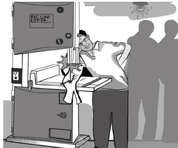
2. Unguarded machines can increase exposure of its moving parts and increase the possibility of accidents.
